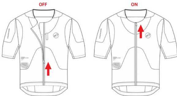
Figure 8: System Turns On When the Activation Zip (2) is Closed
